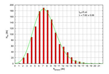
here  $T=5\mu s$ , detector pulse length  $\approx$  18ns, detector dead time  $\approx$  40ns, sampling time bin = 400ps
