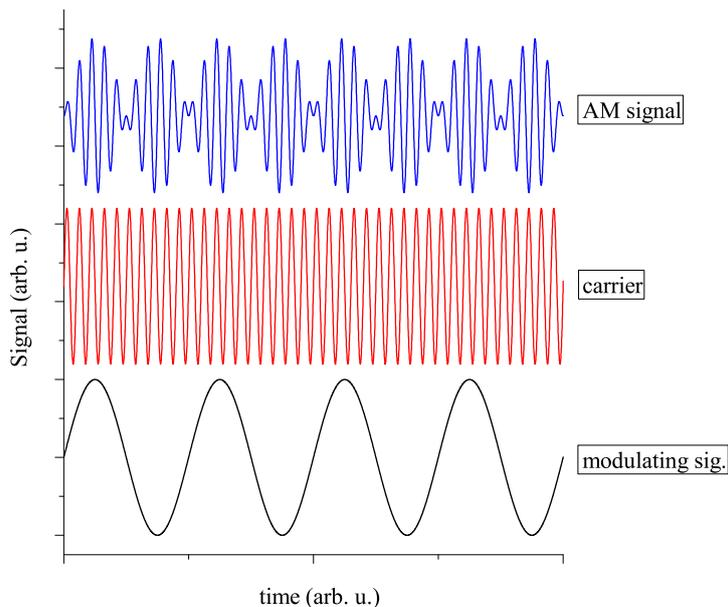
Figure 2.1: Schematics of amplitude modulation.
