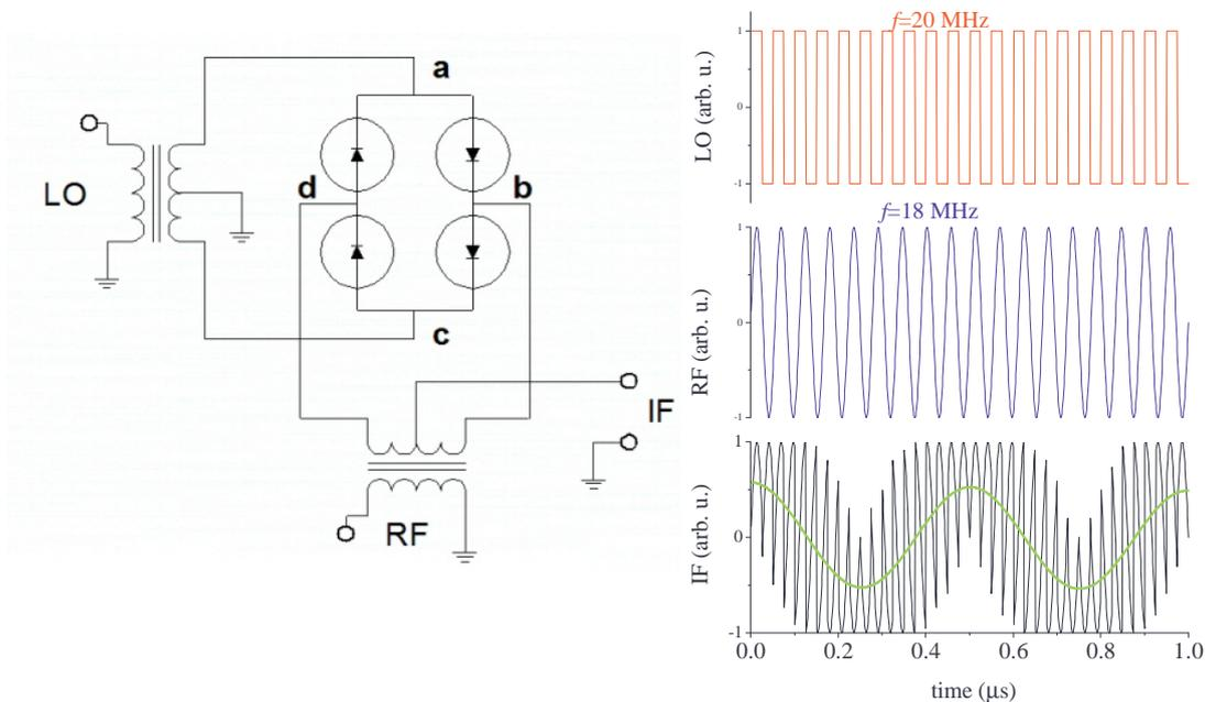
Figure 2.4: Left panel: A possible realization of a mixer, the so-called (switching-mixer). Right panels: the mixer signal for a given example. LO: 20 MHz signal, RF: 18 MHz signal, the IF output is the modulated signal. The green line is the IF signal after low-pass filtering.
