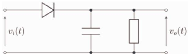
Figure 2.2: Schematics of the detector radio. Input in the left hand-side is rectified and low-pass filtered and arrives to the right hand side output.
