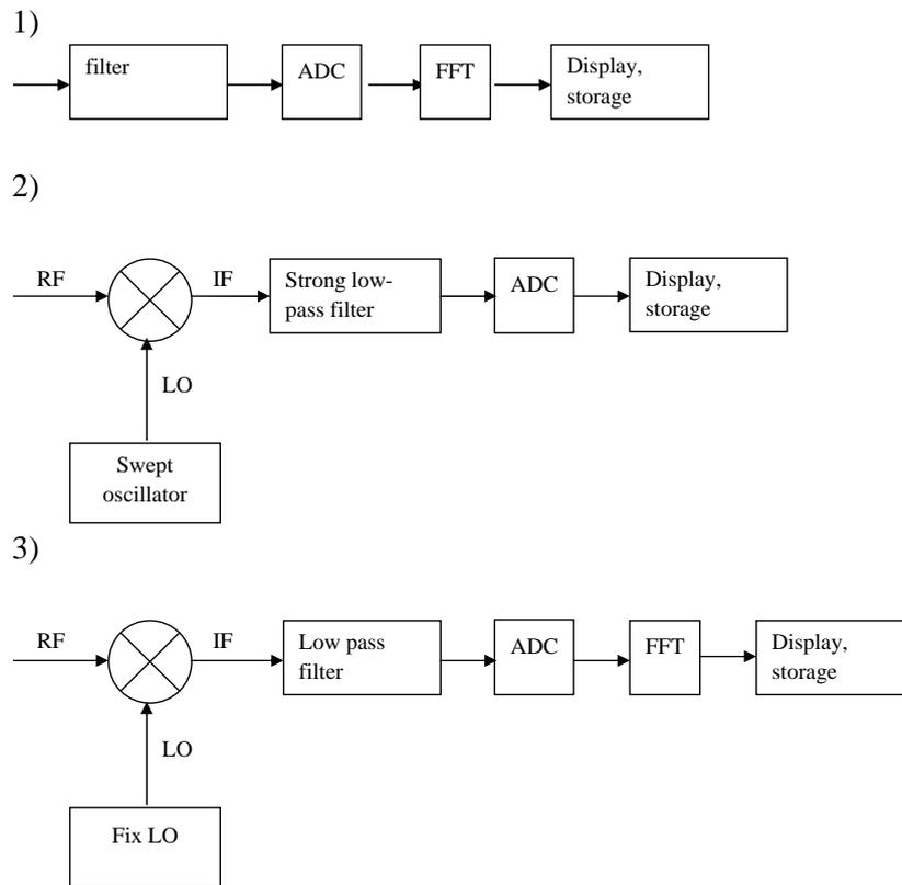
Figure 2.7: Schematics of the three types of spectrum analysis.
