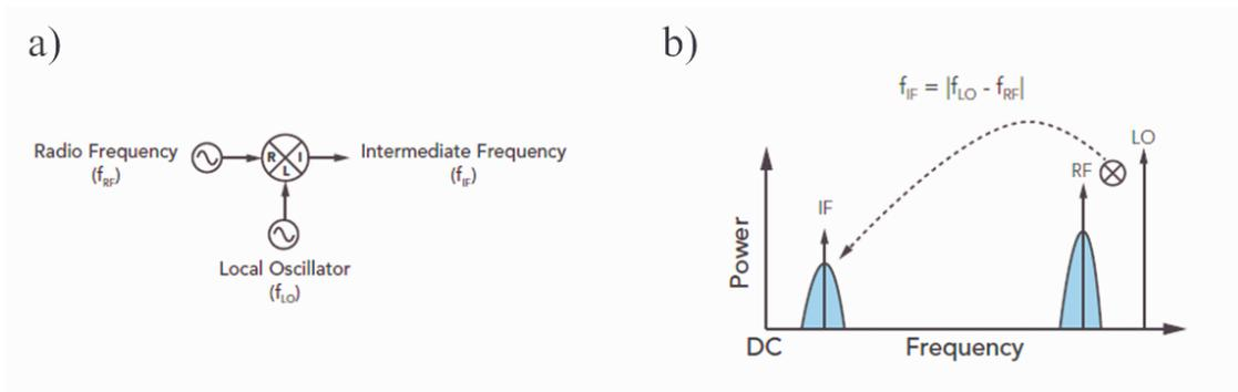
Figure 2.3: a) Mixer symbol with notation of the input-output port: (LO input: local oscillator, RF in/output: radiofrequency signal, IF in/output: intermediate frequency), b) using the mixer as down-converter: IF port is output which has a frequency with the difference of LO and RF.
