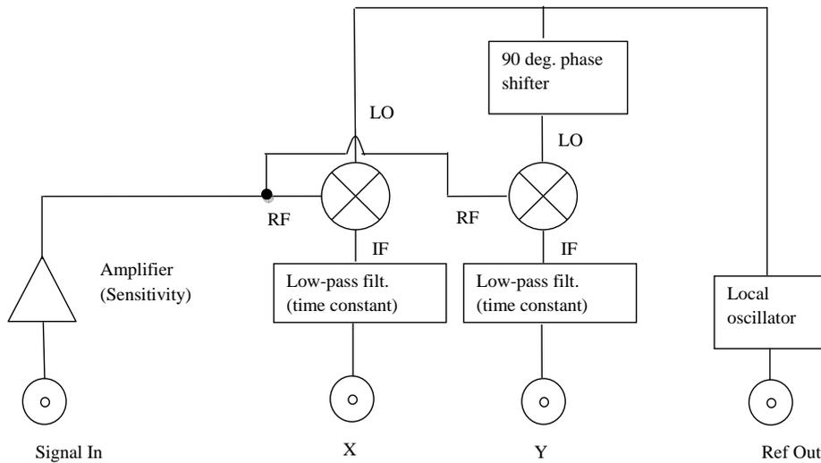
Figure 2.5: Block-diagram of the lock-in amplifier. The layout reflects the control interface of the used Stanford lock-in.
