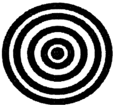
FIG. 5. Fringe pattern of Michelson-interferometer
