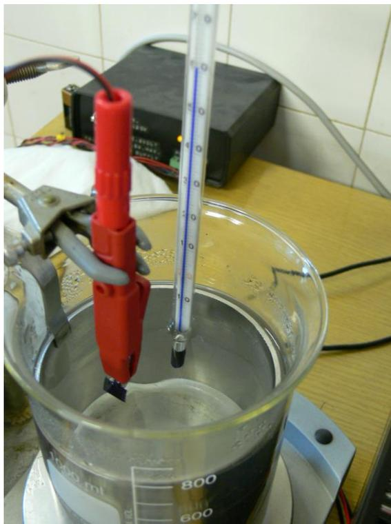
Start the data collection of the oxide growing parameters ( $U_F$ ,  $I_F$ ) by the computer and perform the oxidation successively on all the 3 samples. The oxidation should be carried out until the current decreases below 0,5 mA (i.e. below one tenth of the set current limit).
