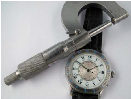
FIGURE 6 The micrometer caliper measures directly a tiny distance or thickness, bypassing x and y coordinates. The watch measures directly the invariant wristwatch time between two events, bypassing separate global coordinate increments. (Photo by Per Torphammar.)
