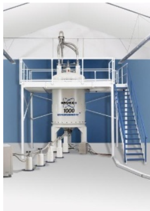
World's first commercial 1000 MHz spectrometer: Bruker Avance 1000 Magnetic field: 23.5 T
